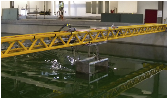
Fig. 3. View of the towing bridge and profile holding structure.
