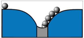
Fig. 2. A schematic of a gravitational analog of the Gaussian gun. A ball released from the left will cause the rightmost ball to be ejected.
