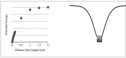
Fig. 4. Potential energy as a function of distance from the magnet (left), and a symmetric potential well based on this data (right).
