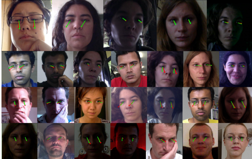
Figure 8: Some prediction results on the MPIIGaze dataset. Green and red lines indicate the predictions and the ground truth, respectively.
