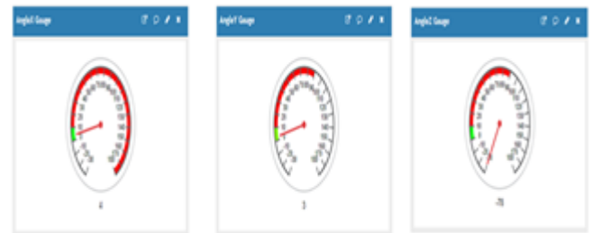
Figure 6. Vibration angle for X, Y, Z when the pantograph touches the NS
