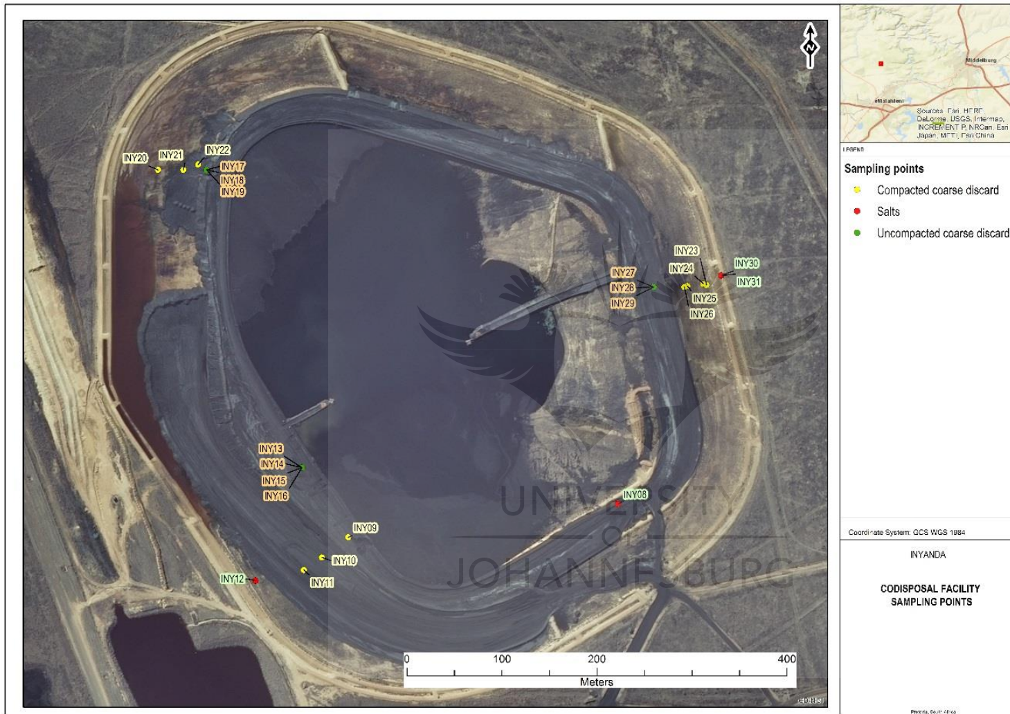
Figure 12 Sample location points at the co-disposal and slurry paddocks facility of the Inyanda coal mine. Adopted from Golder (2015)
