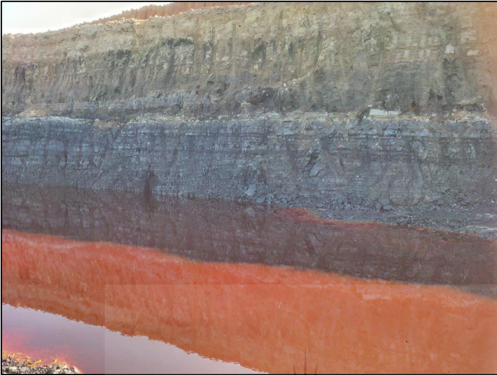
Figure 15: Inyanda Seam 1 and Seam 2 during mining at Pegasus South Pit
