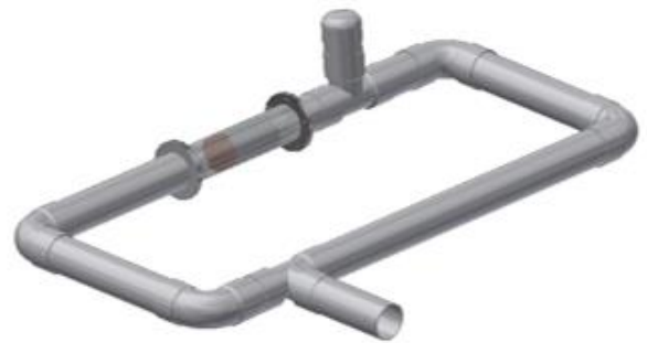
Fig. 7. Looped tube travelling-wave geometry
