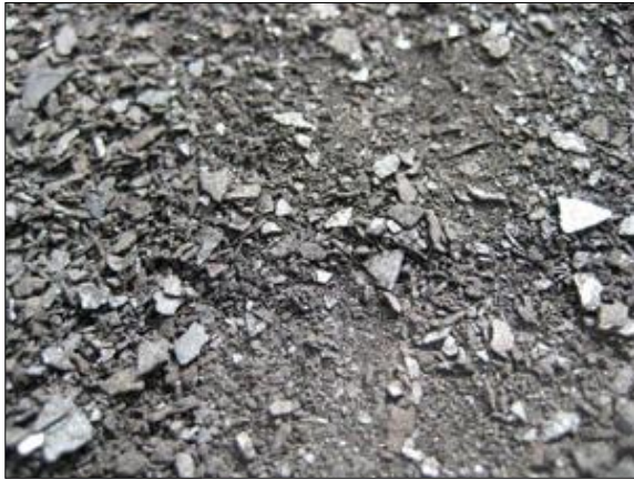
Figure 3-9. Mill scale (NHRTC, 2017)
