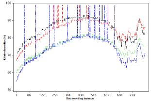
(a) Time series graph of raw relative humidity data (in percentage) recorded by four sensors on the building facade.
