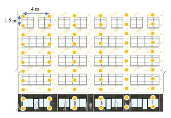
**FIGURE 8.** Suggested sensors' mesh on a simple building facade that was used in Section VII for the creation of a limited digital twin of the building facade.
