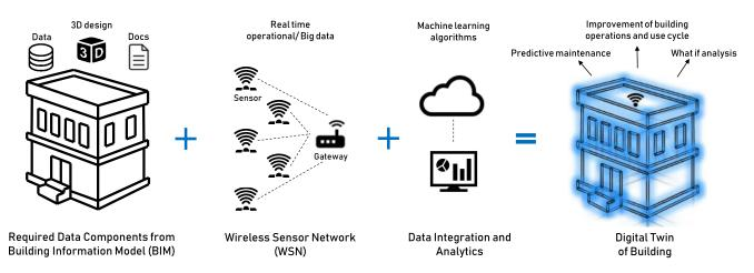
FIGURE 1. Essential components to create a digital twin of building and difference with BIM.
