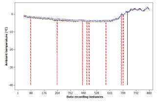
(b) Time series graph of raw ambient temperature data recorded by four sensors on the building facade.
