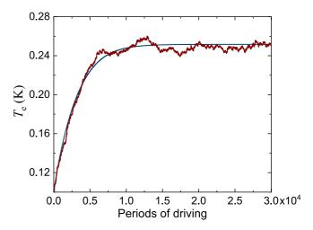
FIG. 4. Long-time behavior of the temperature; the noisy (red) line is a single realization of the qubit-temperature process given by Eqs. (4) and (12) for  $g^2 = 1/100$ . The smooth (blue) line is the evolution of the average temperature by the effective temperature process (27). The parameter values are the same as in Fig. 2.
