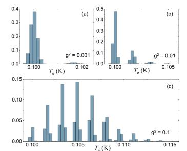
FIG. 2. Temperature distributions after 10 periods of resonant driving for different values of the qubit-calorimeter coupling g. The distributions are obtained from histograms over  $2\times10^5$  realizations. The parameters used for the numerics are  $\hbar\omega_q=k_{\rm B}\times1~{\rm K}, V=10^{-21}~{\rm m}^3, \ \Sigma=2\times10^{-9}~{\rm W~K}^{-5}~{\rm m}^{-3}, \ \gamma=1500k_B/(1~{\rm K}),$  driving coupling constant  $\kappa=0.05$ , and the phonon temperature  $T_p=0.1~{\rm K}$ .
