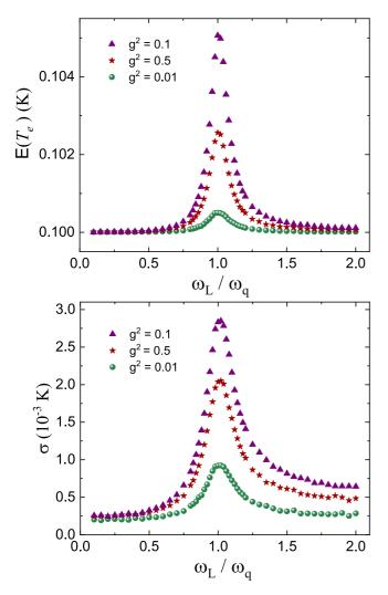
FIG. 3. First moment (top) and the standard deviation (bottom) for the distribution of the temperature after  $10\frac{2\pi}{\omega_q}$  duration of driving. Both the mean and standard deviation peak for resonant driving and higher coupling. The parameters used for the simulations are in the caption of Fig. 2.
