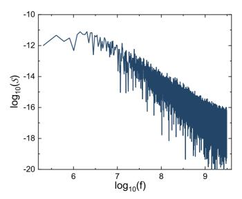
FIG. 8. Power spectrum, for  $g^2 = \frac{10}{100}$ . The spectrum decays with an  $\omega^{-2}$  asymptotic law consistent with the Ornstein-Uhlenbeck approximation (37), (38).
