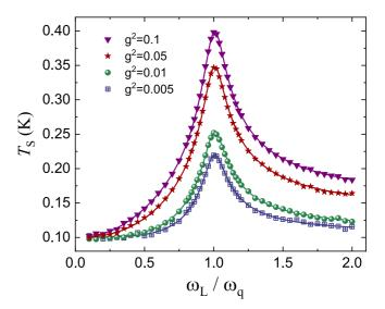
FIG. 5. Mean value of the temperature in the steady state. The data come from a single realization after it reached the steady state as shown in Fig. 4. The full lines are the estimate of the stationary temperature obtained from the solution of (46). The parameter values are the same as in Fig. 2.
