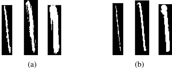
Fig. 4. (a) and (b) Axial micro-CT cross-section images of thresholded images or binary images of the three thickest plates phantom reconstructions correspond to Figure 2(b) and 2(c), respectively.
