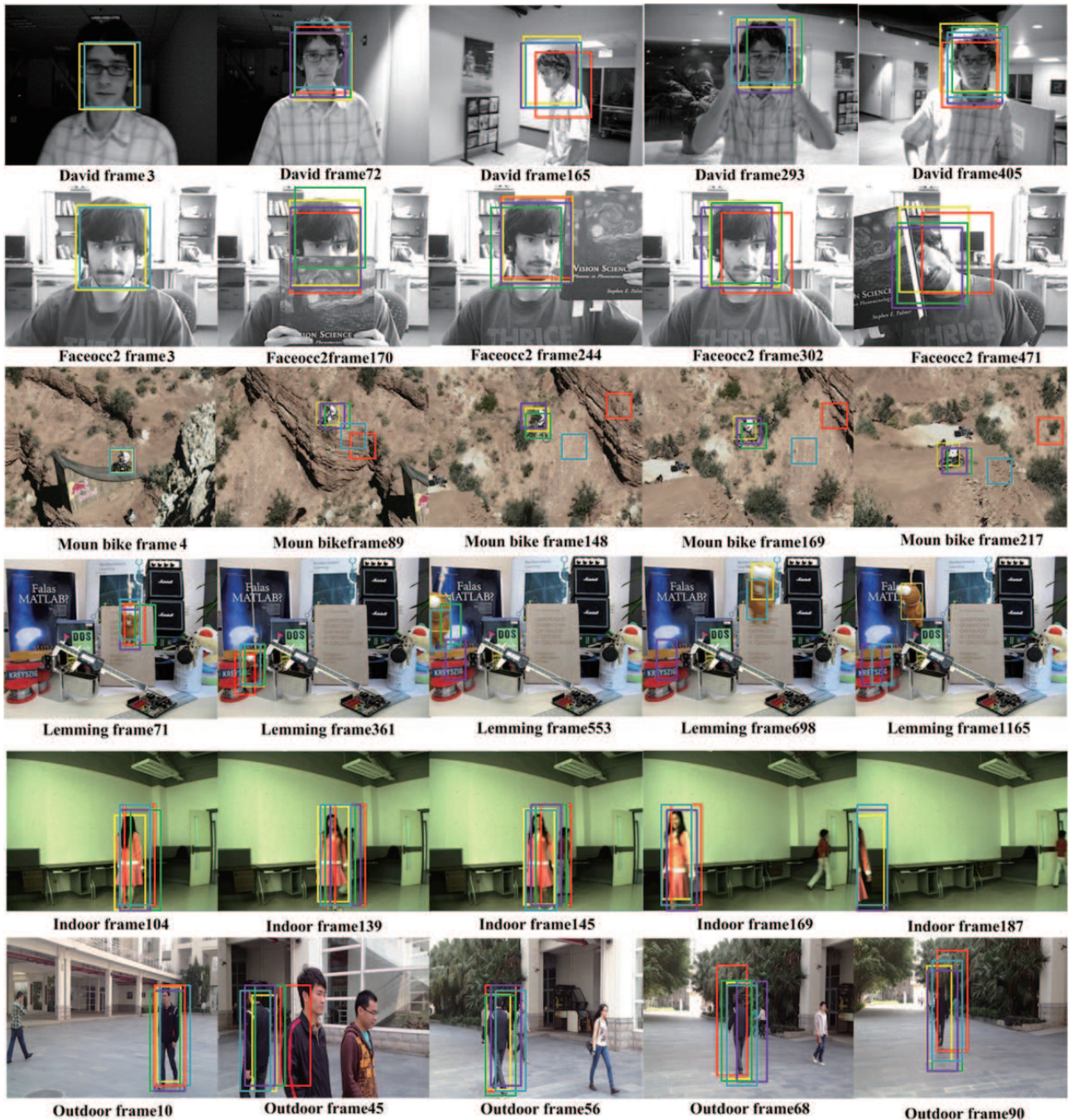
Figure 5. Illustration of tracking results. (Yellow-Ours, Red-OAB, Green-ORE, Purple-HT, Blue-PROST)
