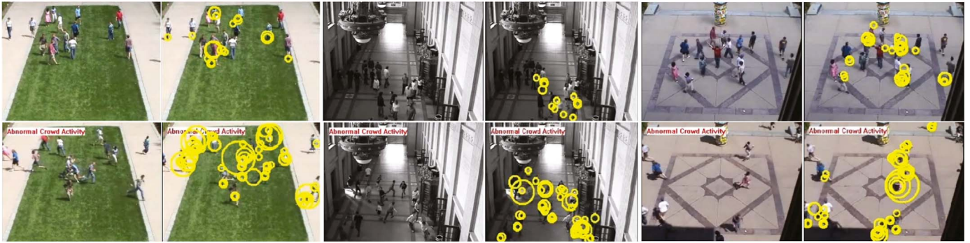
Fig. 8. Three crowd scenes on UMN dataset. Yellow circles represent the local features extracted by Laptev’s detector [41]. Note that the anomaly marks in the second row are from videos. (For interpretation of the references to color in this figure caption, the reader is referred to the web version of this paper.)
