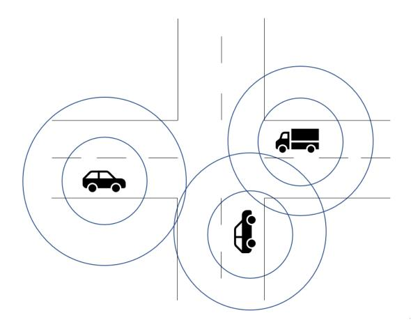
Figure 2.2: Example of an intersection with vehicles working in a Virtual Traffic Light application
