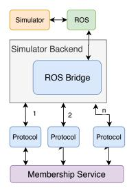
Figure 5.1: Integrated Testing Application Architecture
