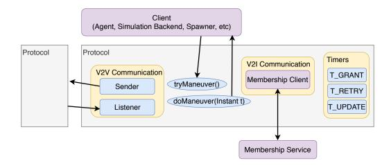
Figure 4.1: Main components of the vehicle coordination protocol implementation
