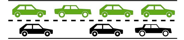
Figure 2.1: Example of a platoon of vehicles (in green) travelling next to regular, noncooperative vehicles (in black)
