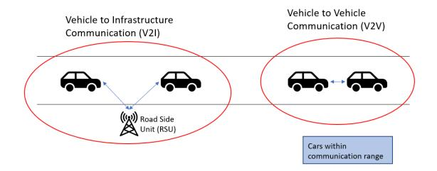
Figure 2.3: Example of vehicles communicating within a VANET
