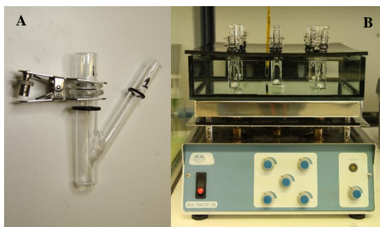
Figure 2.2 - Diffusion studies equipment: Hand-blown Franz-type diffusion cell (A) and the complete experimental apparatus (B), in which 5 diffusion cells are dipped in a thermostatic bath maintained at a constant temperature.
