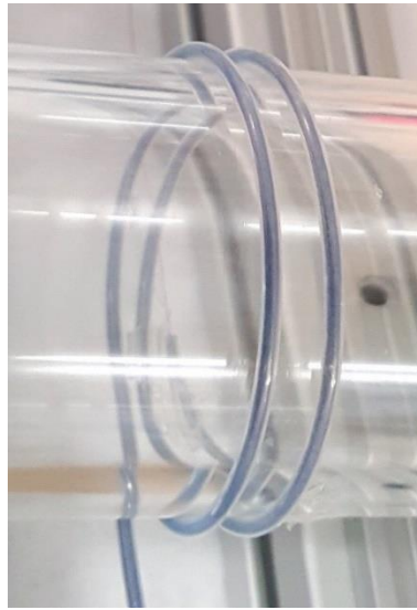
Figure 5. Lubricant experiment. Example of lubricated tube-guided SMA wire actuator. In this case, the guiding tube has been lubricated with fine graphite powder.
