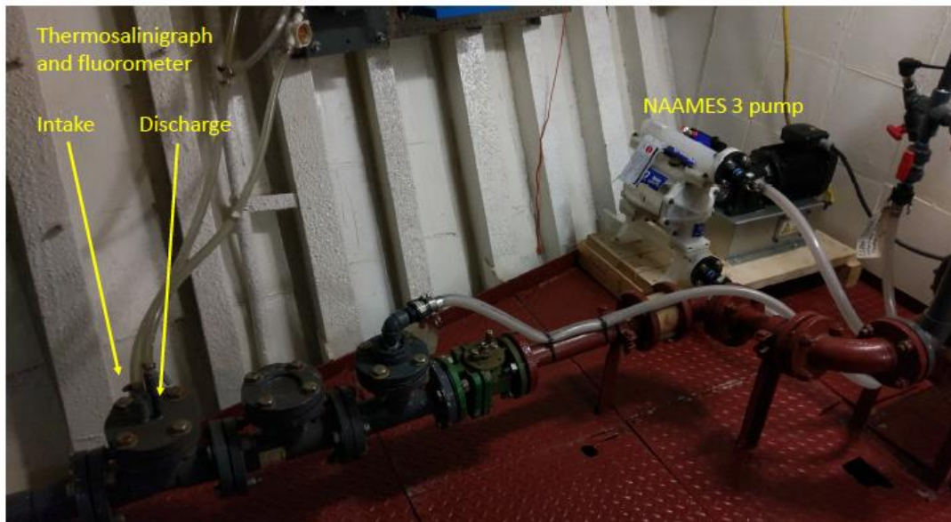
Figure 3. Underway instrument loop and pump on the R/V Atlantis during NAAMES 03.
