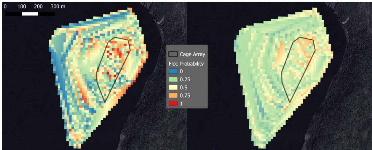
Figure 8. TIN interpolation of predicted probability of flocculent matter presence at Site A. Each map represents the best performing model for each feature set. Left: SMOTE k-nearest neighbor with single beam features only. Right: SMOTE random forest with Boruta selected features.
