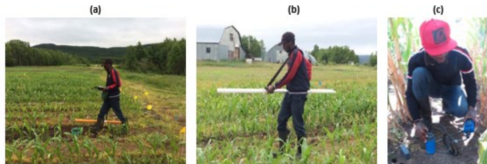
Figure 1.6 Field operation of (a) CMD Mini-explorer (b) GEM-2 (c) HD2-TDR at PBRs, Pasadena, Newfoundland.
