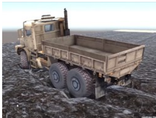
Figure 3-5 Effect of terrain following on the truck movement (AndersOrum, 2015)
