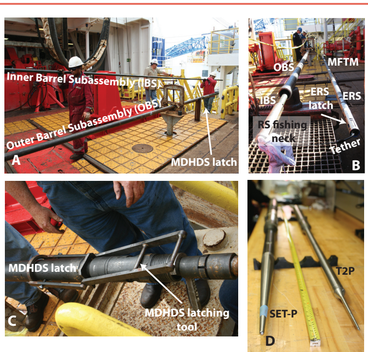
Figure 2. [A] The Inner Barrel Subassembly (IBS) and the Outer Barrel Subassembly (OBS). [B] Left: the IBS lies inside the OBS. The fishing neck of the IBS is shown on the lower left. Right: the ERS is connected to the MFTM, which is connected to the logging line. The ERS Latch is at the bottom of the ERS assembly. [C] The MDHDS Latch and latching tool. The latch is set on the rig floor, and this fixes the IBS to the OBS. When the drillstring is pressurized, this latch is released, and the IBS slides freely from the OBS. [D] The SET-P and the T2P are two pore pressure penetrometers available for use in the drilling program.
