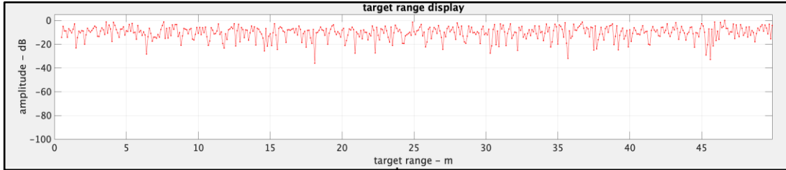
Figure 37: Radar Range profile for Fixed Target SISO -8 dBsm
