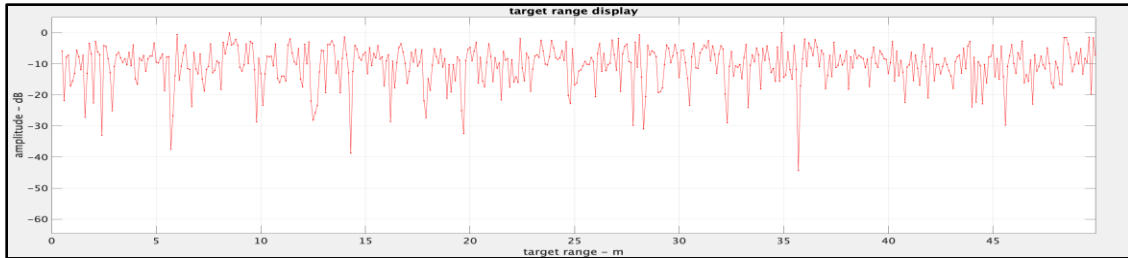
Figure 34: Radar Range profile for Fixed Target SISO 0 dBsm
