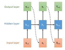
**Figure 5.4:** The Framework of Rnn.  $x_{T-1}$  Represents the Input at Time (T-1). Through Forward Activation, the Input Is Passed Through the Hidden Layers to Generate the Output Where the Error Is Back Propagated to Predict the Correct Output  $y_{T-1}$ . This Output Is Sent along with the Input at Time  $t - x_t$  to Predict the Output  $y_t$
