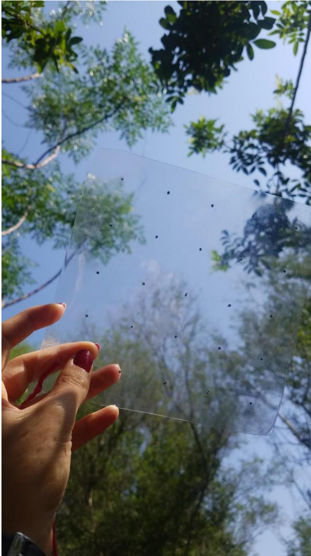
Figure 2a: A canopy scope being used to measure the forest canopy openness. Each dot corresponding to open sky in the largest canopy opening corresponds to 4% canopy openness. Here, five dots correspond to uninterrupted sky which represents 20% canopy openness.
