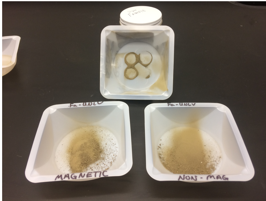
Figure 4.9: The setup used to remove magnetite from the samples. The upper weight boat has several magnets taped to its bottom, and can be seen capturing magnetite grains.
