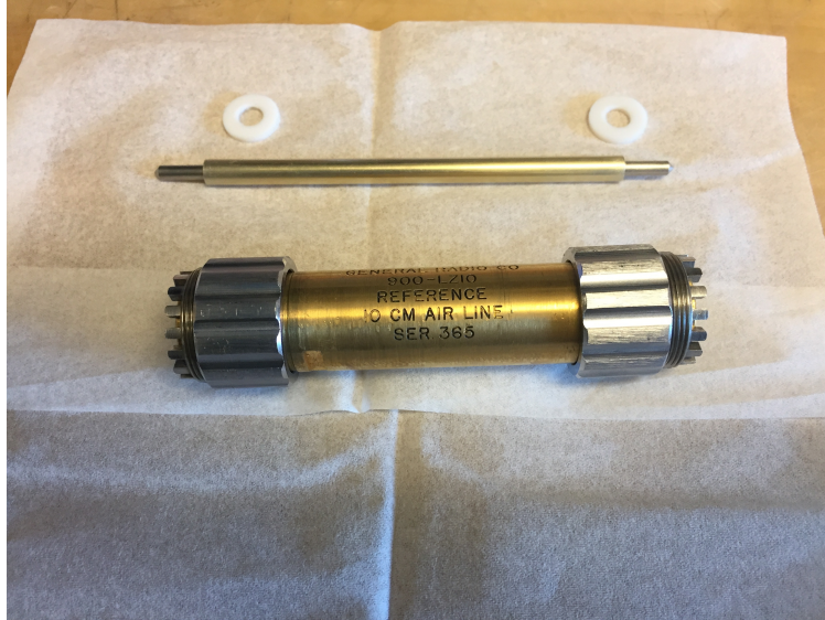
Figure 3.6: 10 cm length GR 900-LZ coaxial airline with inner conductor removed from airline and Teflon ® washers.
