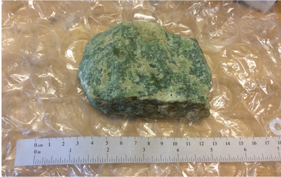
Figure 4.10: Dunite sample provided by the University of Toronto (provenance unknown) that was used in this research.
