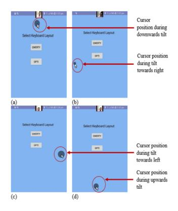
Figure 2.3: (a) EFM cursor position when the device is tilted downwards, (b) EFM cursor position when the device is tilted to the right, (c) EFM cursor position when the device is tilted to the left, (d) EFM cursor position when the device is tilted upwards.
