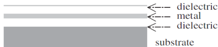
Figure 2-11. Multi-layer coatings design consisting of dielectric/metal/dielectric layers (Reprinted with permission from Ref. [117], The Royal Society).
