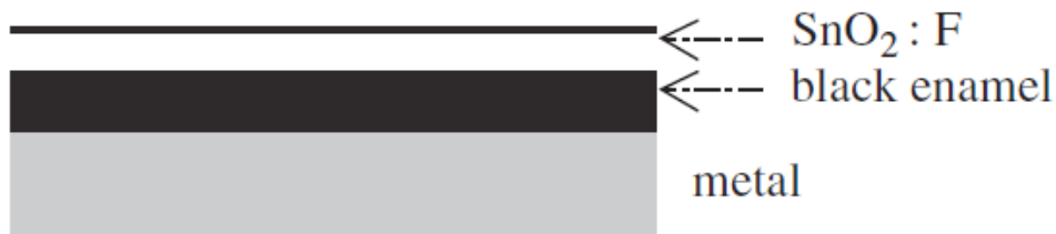
Figure 2-14. A spectrally selective solar-transmitting coating on a blackbody-like absorber (Reprinted with permission from Ref. [117], The Royal Society).
