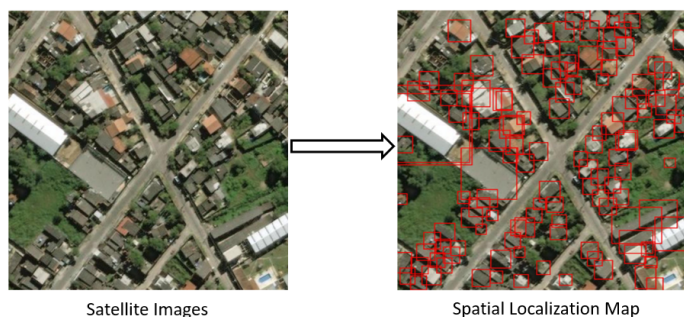
Figure 1.3: Spatial learning: object detection. Red boxes are the bounding boxes of buildings, which describe the building locations.
