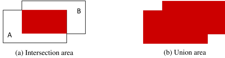
Figure 6.8: Definition of IoU areas, referred as the red regions in the figures.
