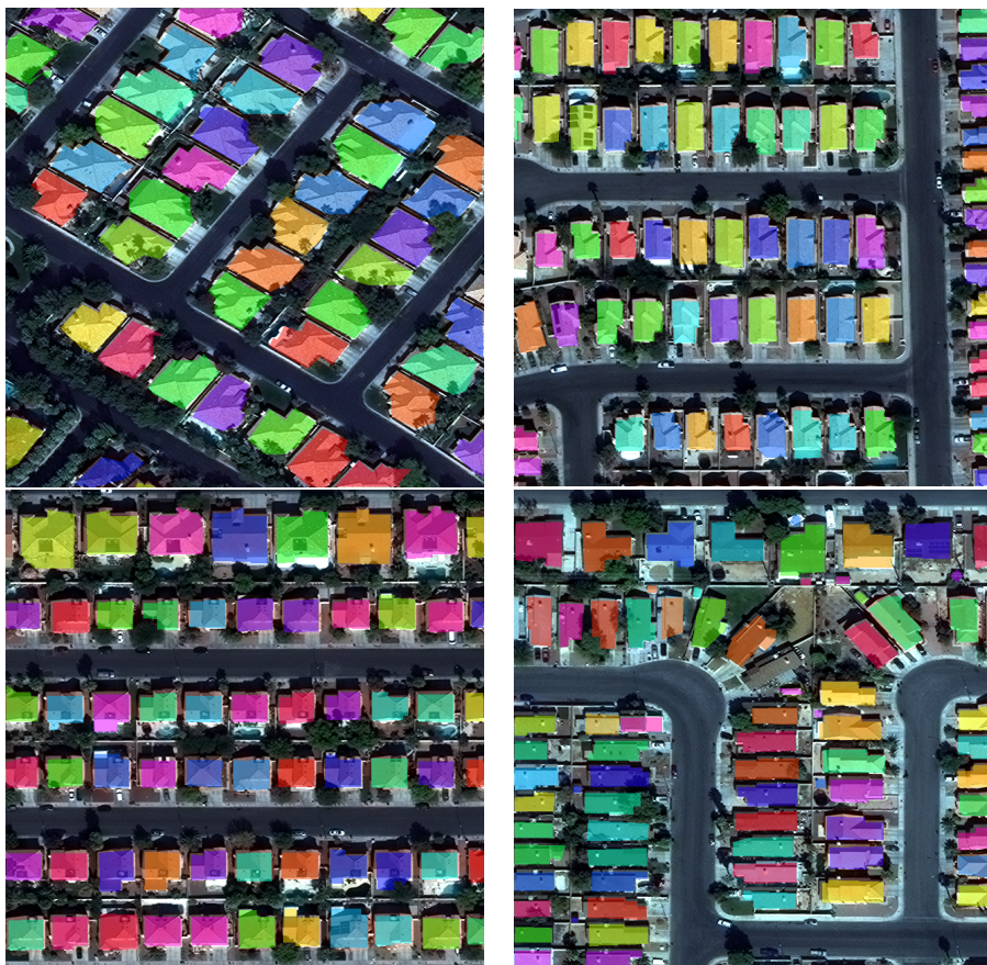
Figure 6.5: Buildings located closely are distinctively detected.
