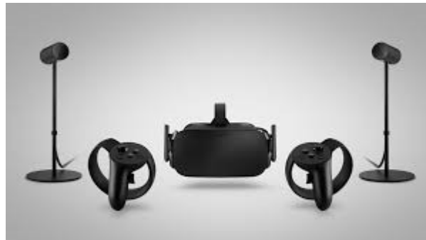
Figure 3.1: Hardware components of oculus rift VR headset
