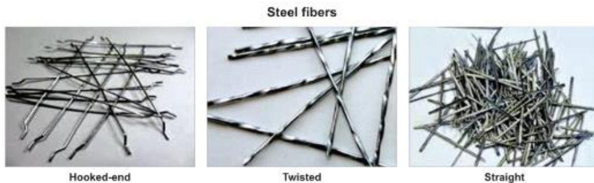
Figure 5.1-2: Examples of Mechanically Deformed Steel Fibers. Reprinted from ‘Ultra High-Performance Fiber-Reinforced Concrete’ by T. Buttignol, J. Souisa, and T. Bittencourt, 2017, p. 961
