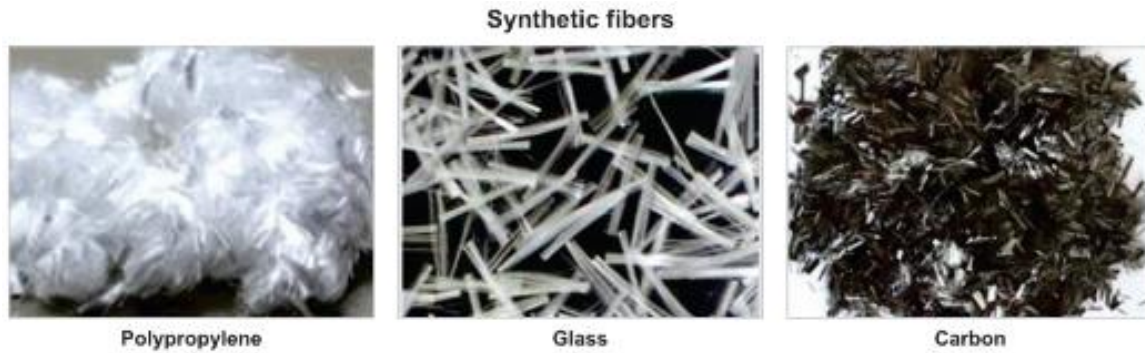
Figure 5.1-1: Examples of Synthetic Fibers. Reprinted from ‘Ultra High-Performance Fiber-Reinforced Concrete’ by T. Buttignol, J. Souisa, and T. Bittencourt, 2017, p. 961
