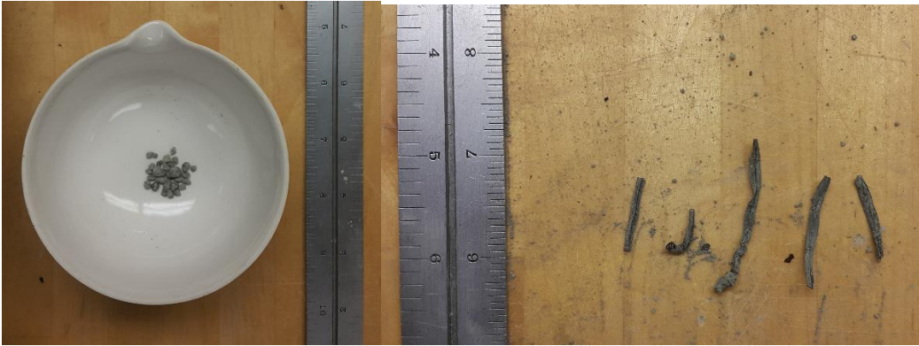
Figure 4.9: (a) Soil Retained on 425- \mu\text{m} (No. 40) Sieve, and (b) Fiber-Like Materials Removed from the Samples
