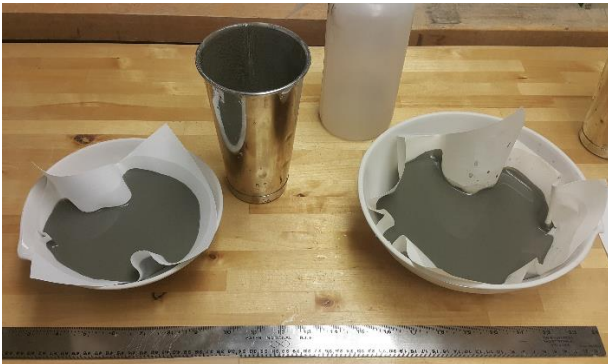
Figure 4.21: Wicking Out the Excess Water from Samples
