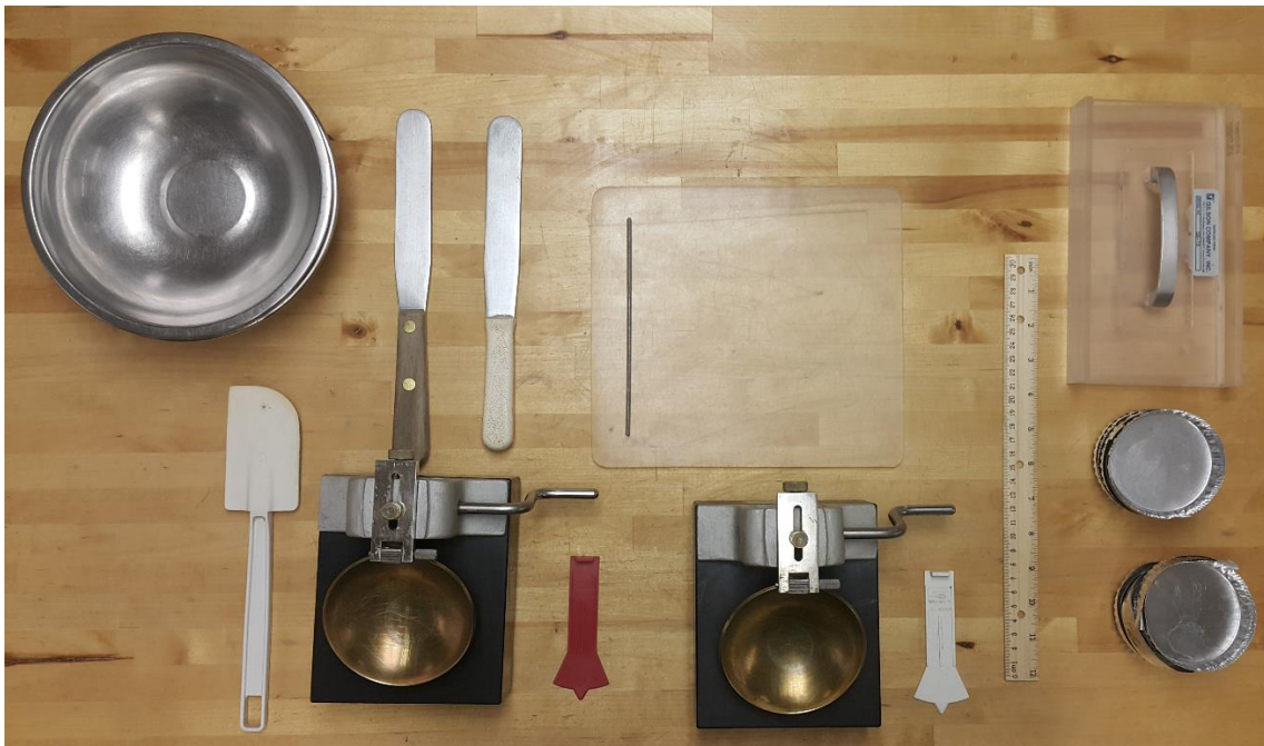
Figure 4.7: Apparatus Used for Liquid Limit, Plastic Limit, and Plasticity Index Tests
