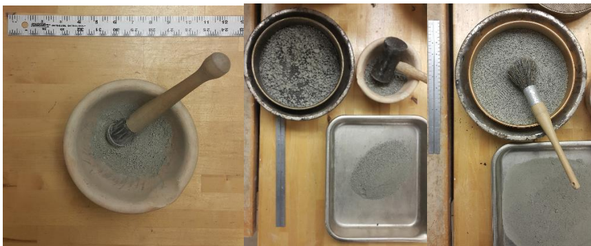
Figure 4.6: First Pulverization of the Obtained Samples
