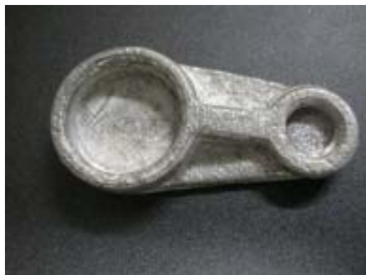
Fig. 9 A pure aluminum casting work piece
