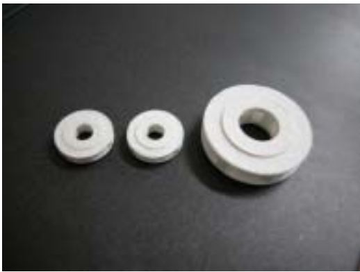
Fig. 5 Pump blades made of ceramic
