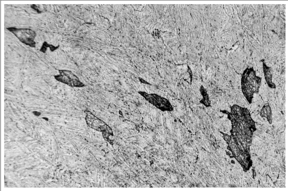
Figure 5 - Optical Micrograph Showing Local Inhomogeneities
