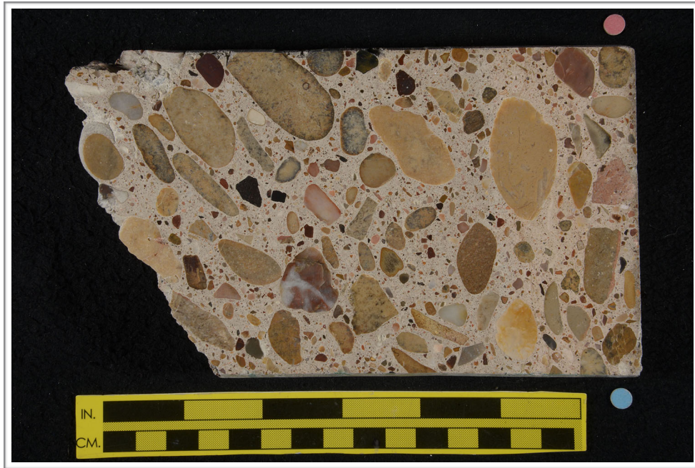
Figure A2. Photograph showing the polished surface of the core. The large and small divisions on the yellow scale are in inches and centimeters, respectively.
