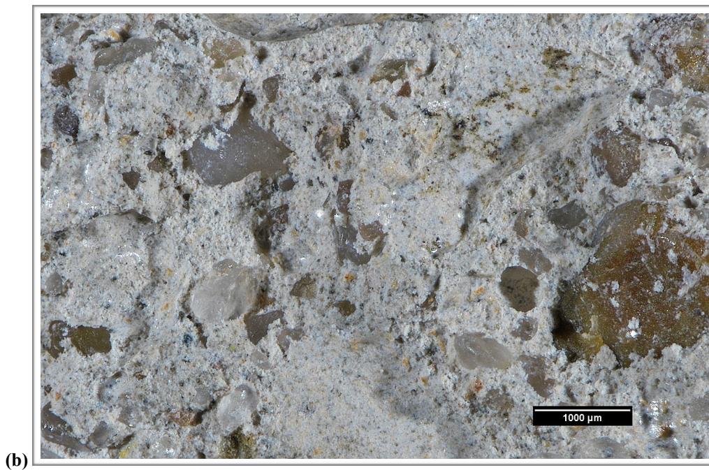
Figure B9. (a) Photograph and (b) reflected light photomicrograph of fresh fracture surface. The scale is in millimeters in (a).
