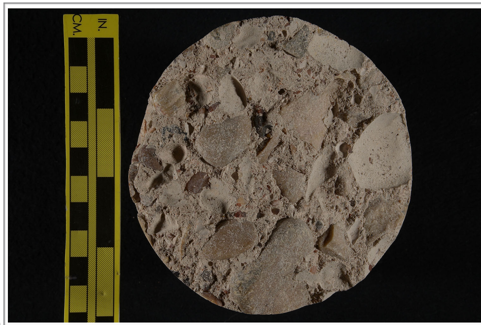
Figure A1 (cont'd). Photographs of the core in as-received condition showing the (c) side of the core and (d) the inner surface of the core. The yellow scale in (c) is ~ 150 mm (6 in.) long; the large and small divisions on the yellow scale in both photos are in inches and centimeters, respectively.
