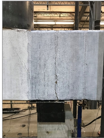
d) CFRP retrofitted span after test completion (west face)
