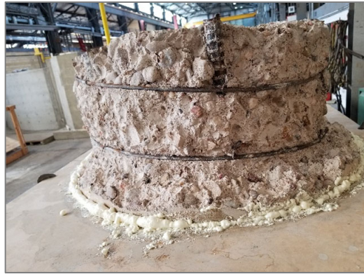
(b) Column stub with perimeter-enclosing fibreboard and removed concrete cover
