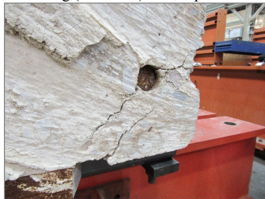
f) Pullout of bottom longitudinal bar after test completion
