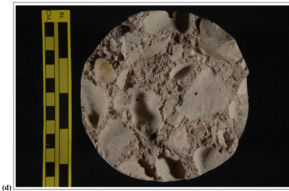
Figure B1 (cont'd). Photographs of the core in as-received condition showing the (c) side of the core and (d) the inner surface of the core. The yellow scale in (c) is ~ 150 mm (6 in.) long; the large and small divisions on the yellow scale in both photos are in inches and centimeters, respectively.
