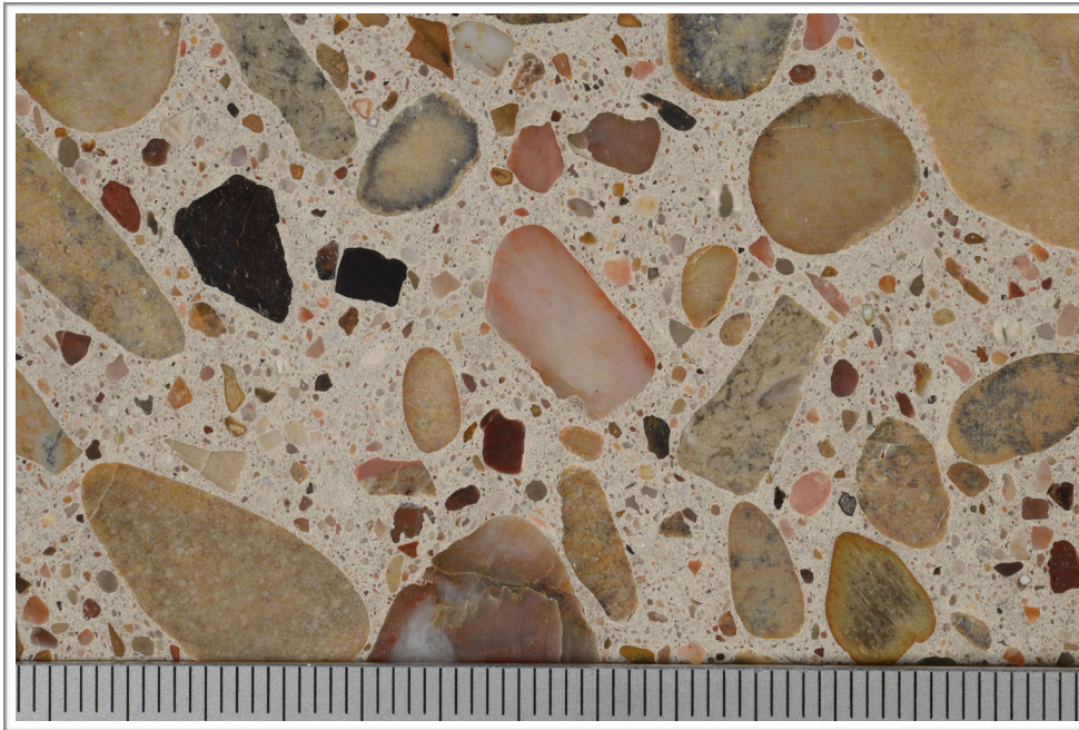
Figure A6. Photograph of the polished surface showing overview of coarse aggregate; scale in millimeters.
