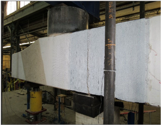
a) Formation of major flexural and shear cracks (west face)
