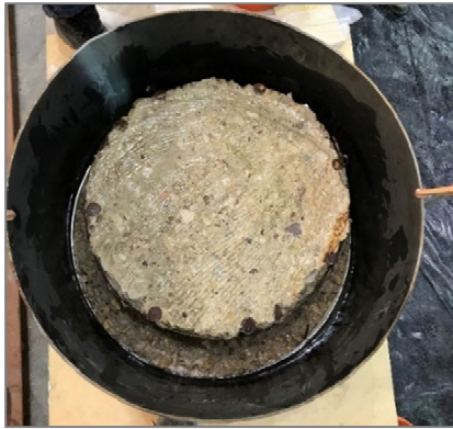
(c) Steel jacket enclosing column stub
