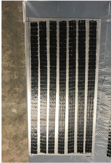
(b) CFRP coupons showing 3 unidirectional strips per specimen
