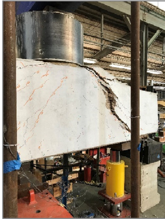
e) Shear cracks at overhang after test completion (west face)
