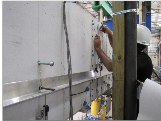
b) Crack width measurements
