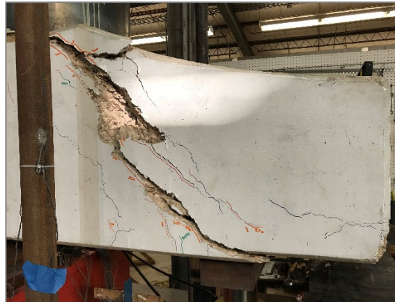
f) Shear cracks and concrete crushing at overhang after test completion (west face)
