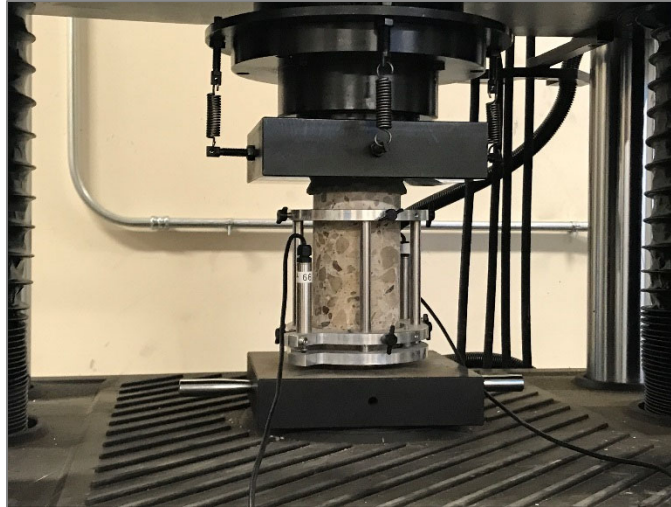
Figure 2.13. Compression test setup on the MTS universal testing machine
