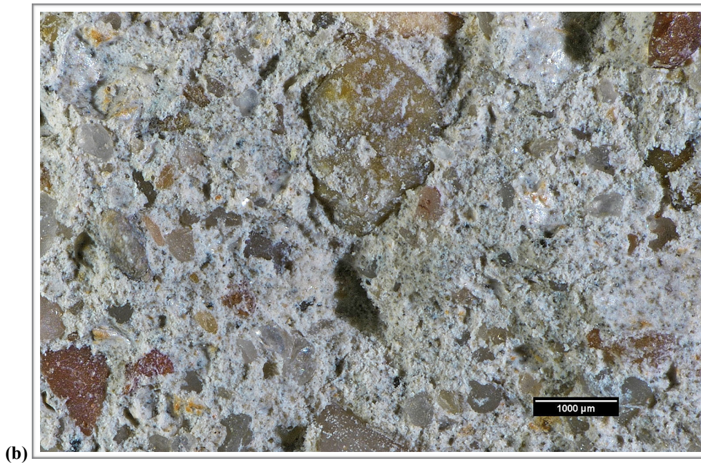
Figure A9. (a) Photograph and (b) reflected light photomicrograph of fresh fracture surface. The scale is in millimeters in (a).
