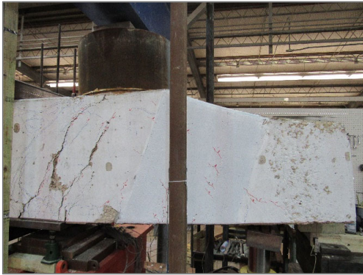
c) Shear cracks after cap failure (west face)
