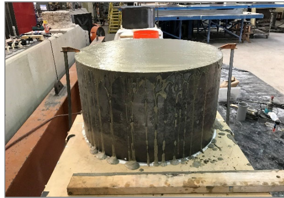
(d) Finished column stub with finished top surface
