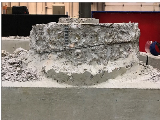
(a) concrete cover removal from BC1 middle column stub
