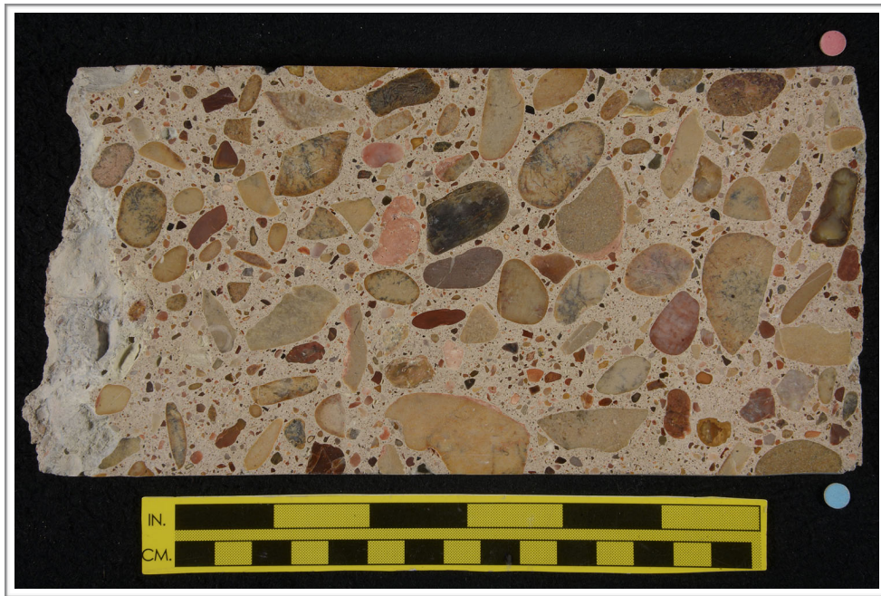
Figure B2. Photograph showing the polished surface of the core. The large and small divisions on the yellow scale are in inches and centimeters, respectively.
