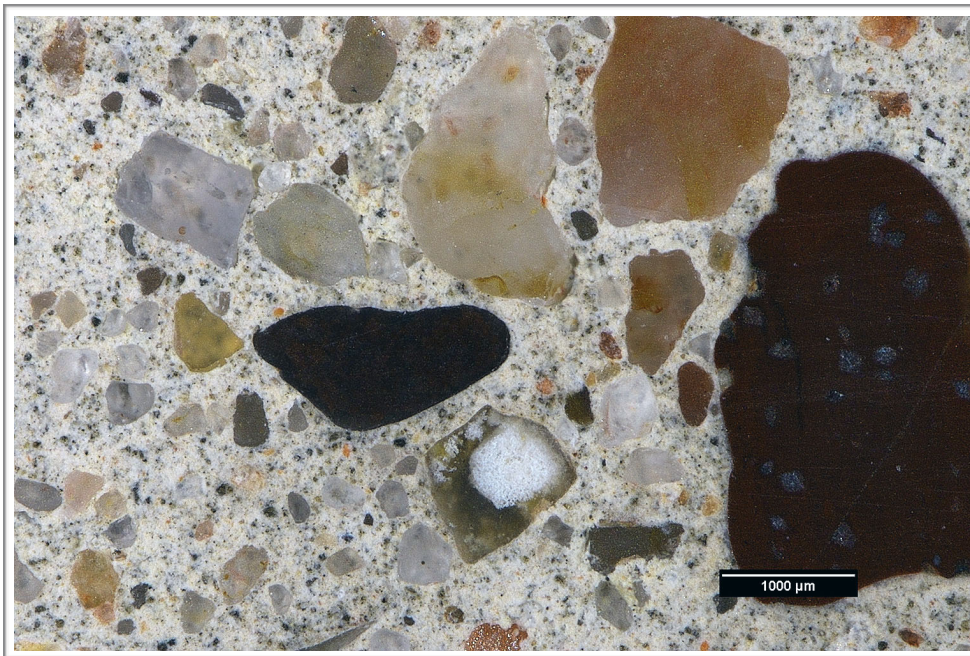
Figure A7. Reflected light photomicrograph of the polished surface showing the fine aggregate.
