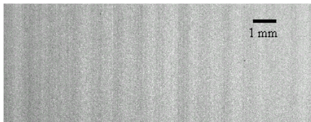
Figure 5. Top surface of jetted bed, typical region. 18 vol % slurry.
