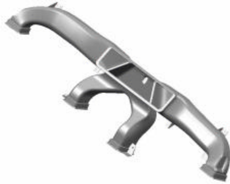
Fig. 2 Feature of heater to air ventilation duct connector
