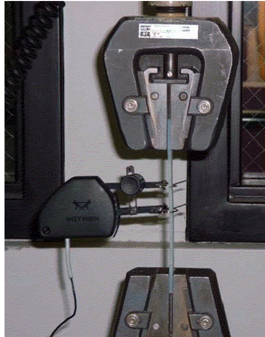
Figure 4: Instron tensile testing set-up
