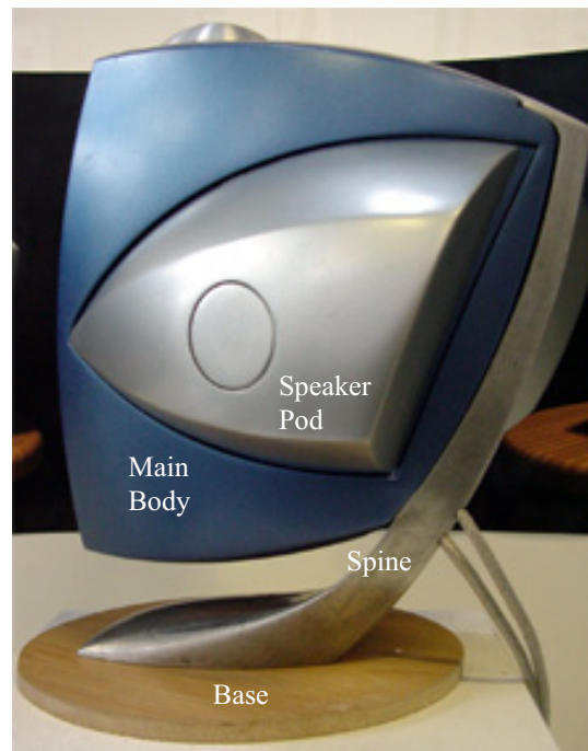
Figure 6: CD Player with various features indicated.
