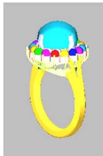
(b) Multi-colour STL model modified from monochrome STL model
