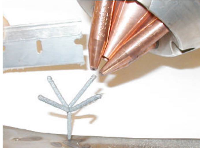
Figure 15. A branched structure made by laser cladding
