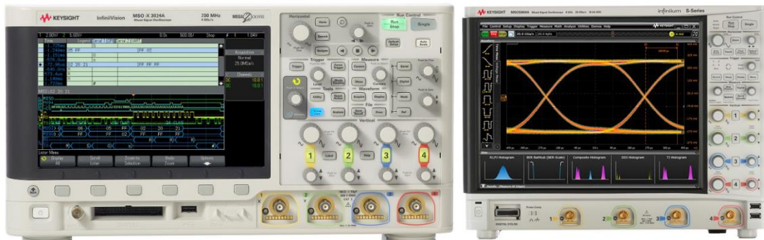
Figure 7: Keysight’s Infiniivision scope [25] (left) performs a single measurement in every acquisition cycle while the Infiniium scope [26] (right) captures up to 4096 signals per acquisition cycle making experiments significantly faster.
