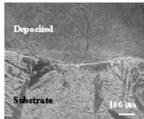
Fig. 9 Interface between the substrate and the deposited wall
