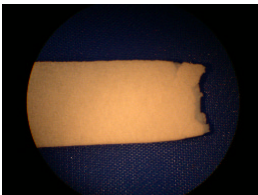
Figure 8A. Duraform PA Nylon Necking
