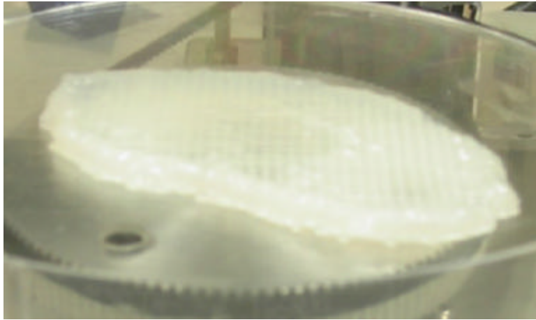
(c) Scaffold part built (15 layers)
