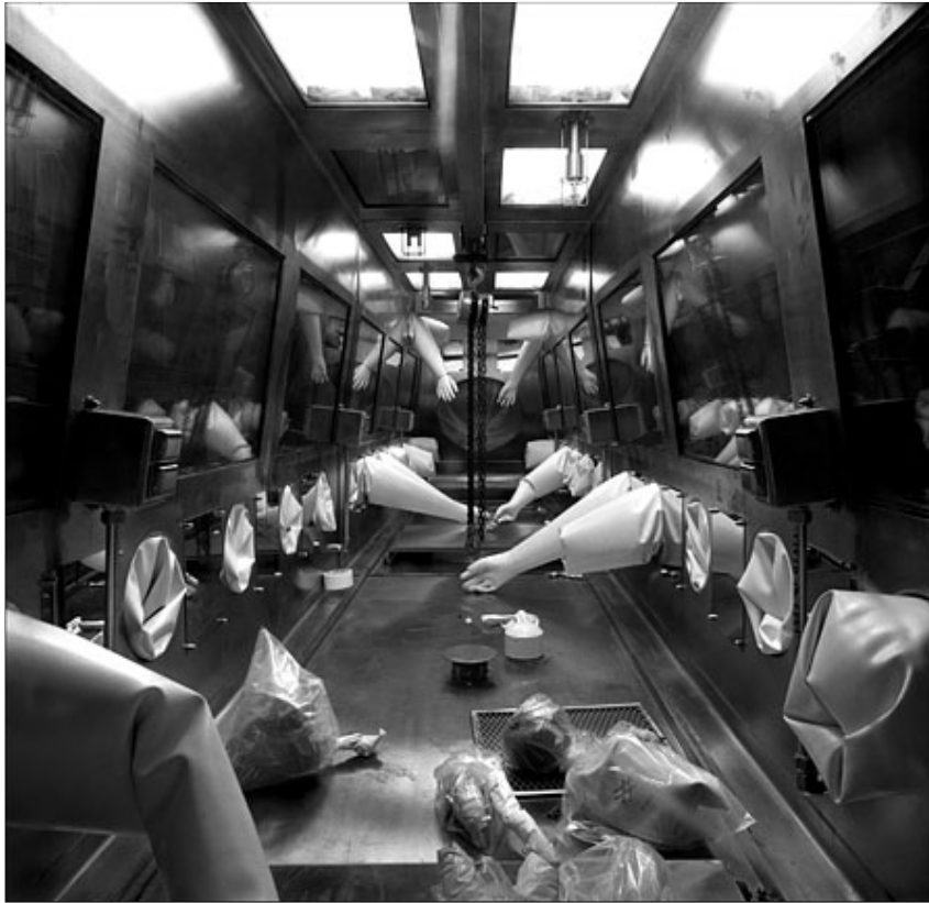
Figure 1.1: A glovebox as used in the nuclear industry at the Rocky Flats Nuclear Weapons Plant [42].
