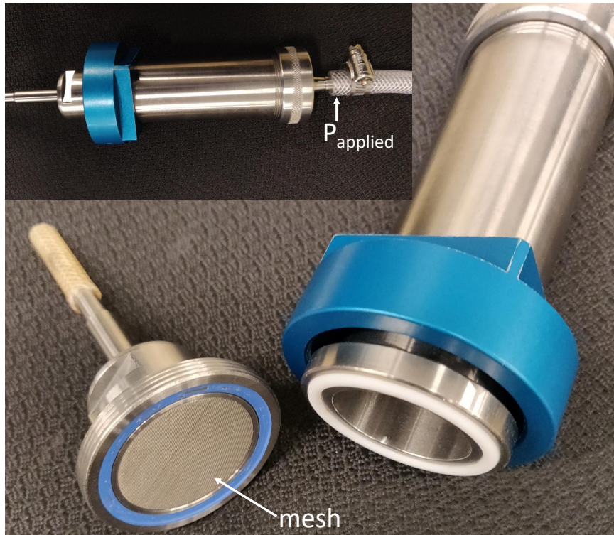
Figure 4.2: Experimental set up used to measure Darcy permeability.
