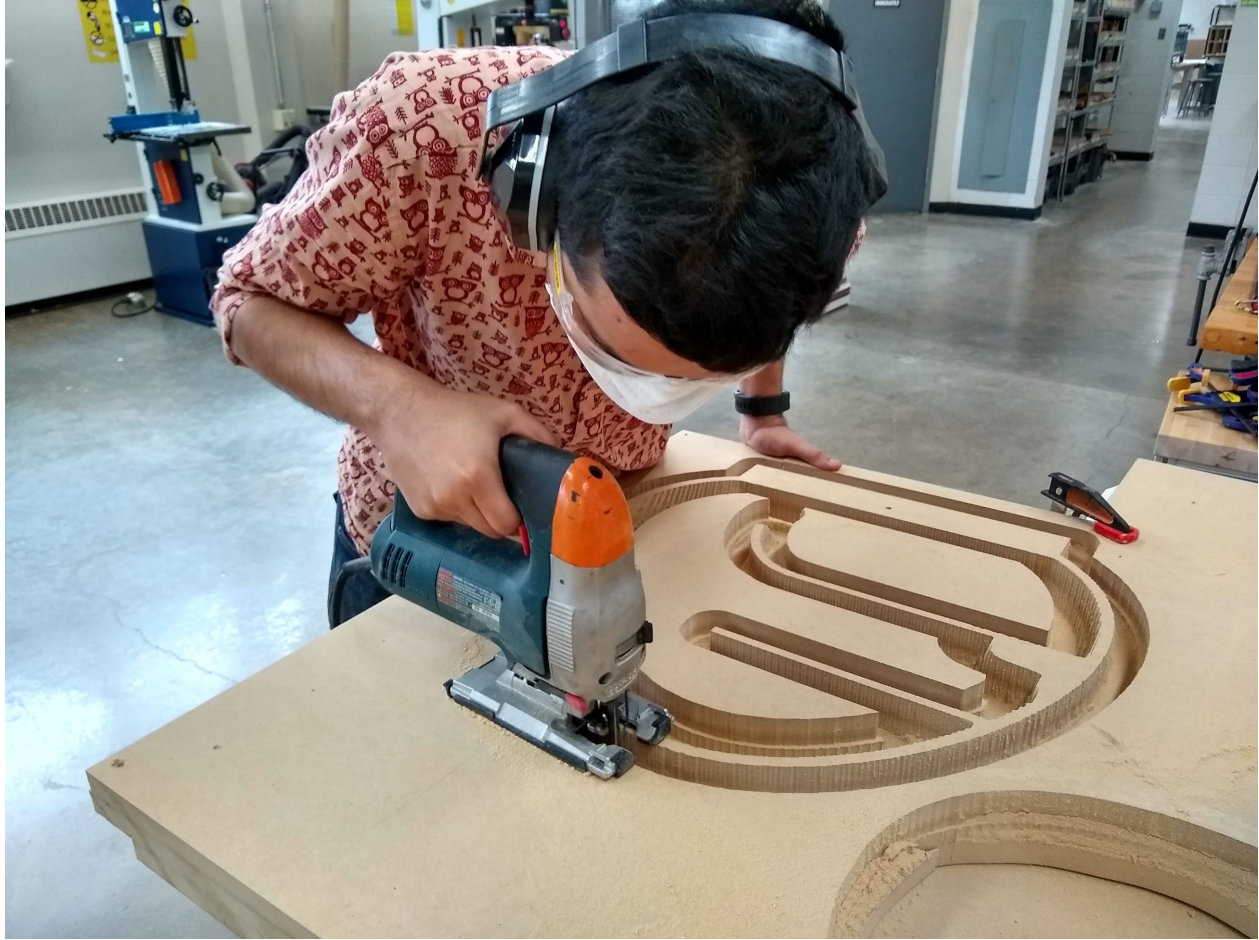
Figure 6.3: Pieces separated using a jigsaw
