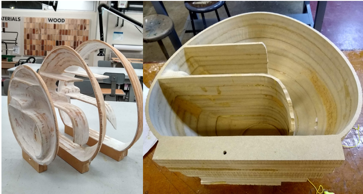
Figure 6.4: Blocks sanded and glued up
