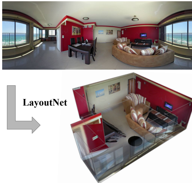
Figure 3.1: Illustration. Our LayoutNet predicts a non-cuboid room layout from a single panorama under equirectangular projection.
