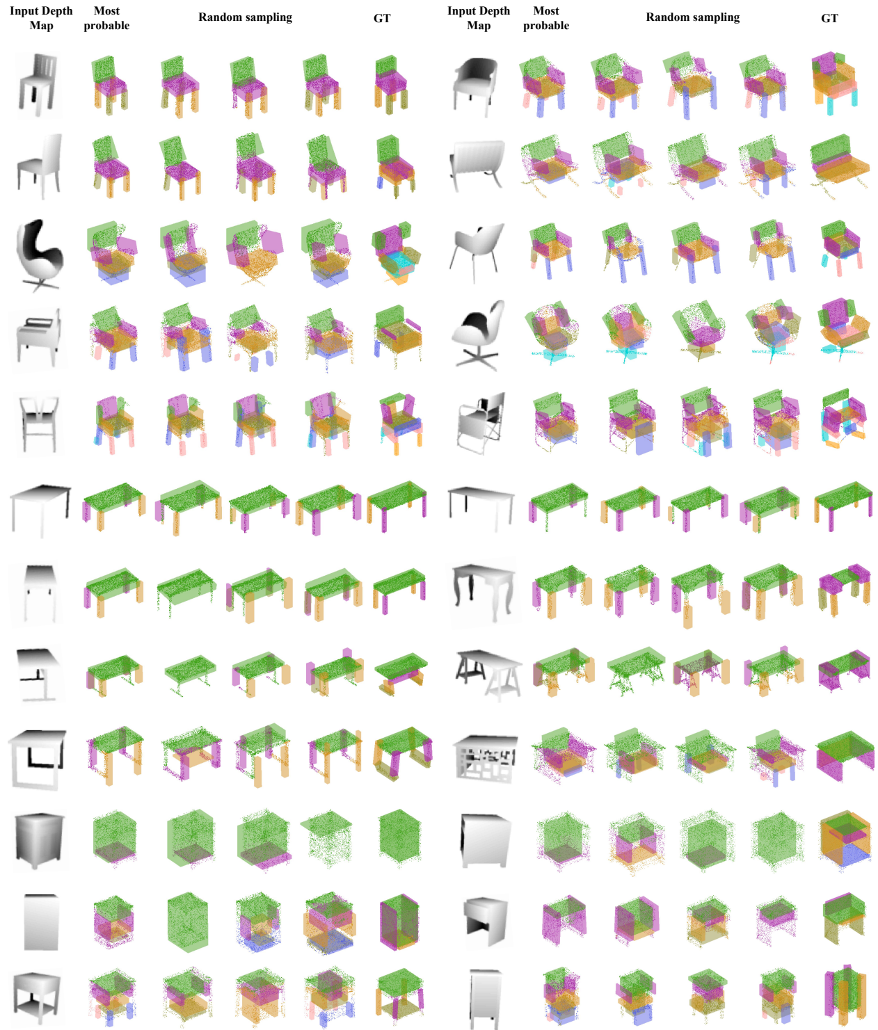
Figure 6.8: Sample reconstruction from synthetic data from ShapeNet. We show the input depth map, with the most probable shape reconstruction from 3D-PRNN, and three successive random sampling results, compared with our ground truth primitive representation. Better view in color.
