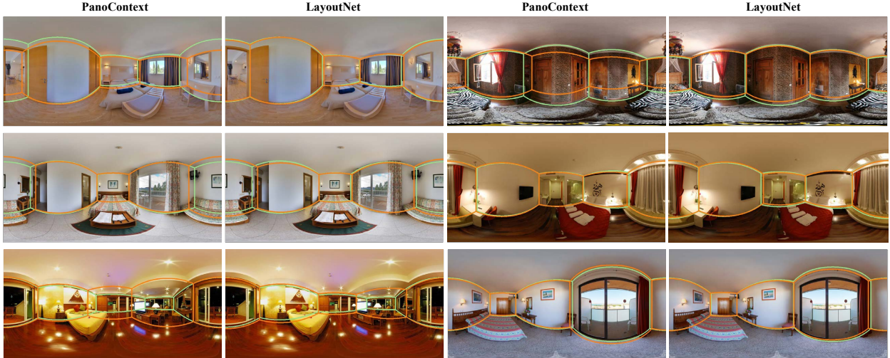
Figure 3.3: Qualitative results (randomly sampled) for cuboid layout prediction on PanoContext dataset. We show both our method’s performance (even columns) and the state-of-the-art [31] (odd columns). Each image consists predicted layout from given method (orange lines) and ground truth layout (green lines).
