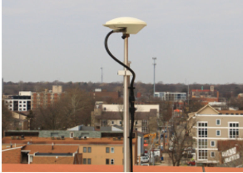
Figure 6.1: Rooftop antenna setup in Urbana, Illinois
