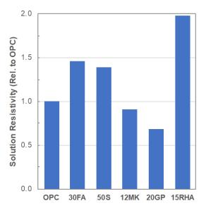
**Fig. 4.** Relative pore solution resistivity, as measured for solutions extracted from cement pastes after one year of curing
