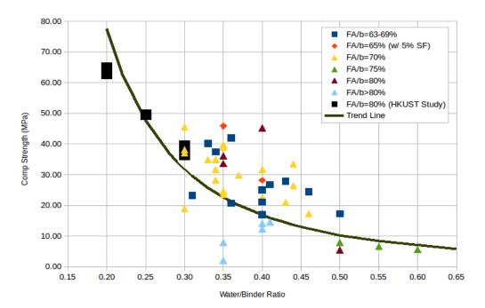
Fig 14. Compressive strength of high volume fly ash green concrete (Yu et al., 2017b).
