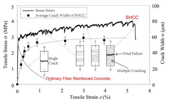
Fig 7 Typical tensile stress-strain behaviour of a green HVFA-SHCC (Adapted from Li, 2012).
