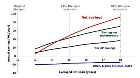
**Fig 10.** Graphs showing net savings over the life cycle of a typical asphalt road surface in Netherlands by use of self-repairing porous asphalt concrete (NL Agency, 2011)
