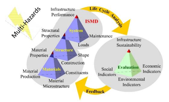
**Fig 6**. Integrated materials design framework for sustainable infrastructure combining Performance Driven Design Approach (PDDA) (Li, 1992) & Integrated Structures and Materials Design philosophy (ISMD) (Lepech, 2011).
