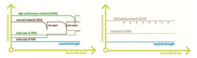
Fig. 12. Schematic of service life of concrete structure with self-healing (Sangadji, 2015)
