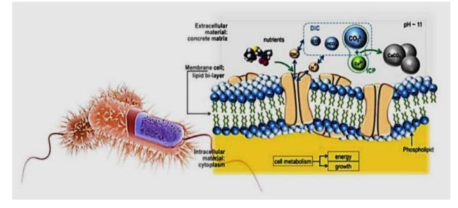
Fig 4. Working mechanism of bio-based concrete healing developed by Microlab (Sangadji, 2015)
